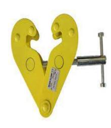
URBANLIFT CLAMP beam clamp provides a quick and versatile rigging point for hoisting equipment, pulley blocks or loads and comes complete with a locking device. The unit offers flexible applications, due to the wide adjustment range. The central threaded spindle allows easy attachment and a safe and secure grip to the beam flange.
